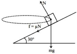
At  $v_{max}$ , f will be limiting in nature.  $\therefore$  Balancing force in vertical direction,  $N \cos 30^\circ - mg - \mu N \cos 60^\circ = 0$   $\Rightarrow N \left[\cos 30^\circ - \mu \cos 60^\circ\right] = mg$   $\therefore N = \frac{800 \times 10}{(0.87 - 0.1)} \approx 10.2 \times 10^3 \text{kgm} / \text{s}^2$ Hence option 1.
