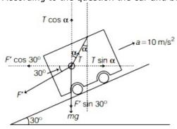
Here, F' is the pseudo force acting on the bob when we considered it from car's frame and T is the tension on the string. In equilibrium,  $\Sigma F_x = 0$  and  $\Sigma F_v = 0$
