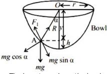
mgThe insect crawls up the bowl upto a certain height honly till the component of its weight along the bowl is balanced by limiting frictional force.
