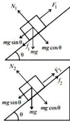
When the body slides up the inclined plane, then
