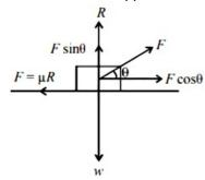
For horizontal equilibrium,  $F \cos\theta = \mu R ......(i)$  For vertical equilibrium,  $R + F \sin\theta = mg$  or,  $R = mg - F \sin\theta ......(ii)$  Substituting this value of R in eq. (i), we get  $F \cos\theta = \mu(mg - F \sin\theta) = \mu mg - \mu F \sin\theta$  or,  $F (\cos\theta + \mu \sin\theta) = \mu mg$  or,  $F = \frac{\mu mg}{\cos\theta + \mu \sin\theta} ......(iii)$
