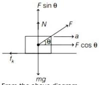
From the above diagram,  $N = mg - F \sin \theta...(i)$  where, N = normal force and  $F \cos \theta - f_k = ma$   $\Rightarrow F \cos \theta - \mu_k N = ma ...(ii)$  where,  $f_k = \text{kinetic friction force}.$  From Eq. (i) and Eq. (ii), we get  $F \cos \theta - \mu_k (mg - F \sin \theta) = ma$   $\Rightarrow a = \frac{F}{m} \cos \theta - \mu_k \left(g - \frac{F}{m} \sin \theta\right)$
