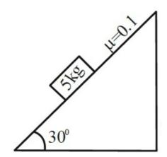
If  $\overrightarrow{F}_1$  is the force required to just move the block up the inclined plane and  $\overrightarrow{F}_2$  is the force required to just prevent the block from sliding down, then the value of  $|\overrightarrow{F}_1| - |\overrightarrow{F}_2|$  is : [Use g=10m/ s<sup>2</sup>]
